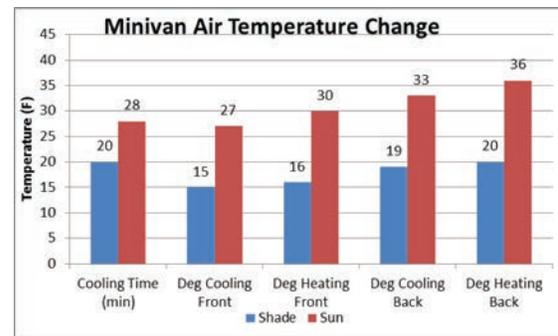
**Figure 5** – Average cooling time and temperature changes.
