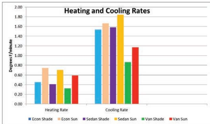
Figure 4 – Average heating and cooling rates of vehicles
