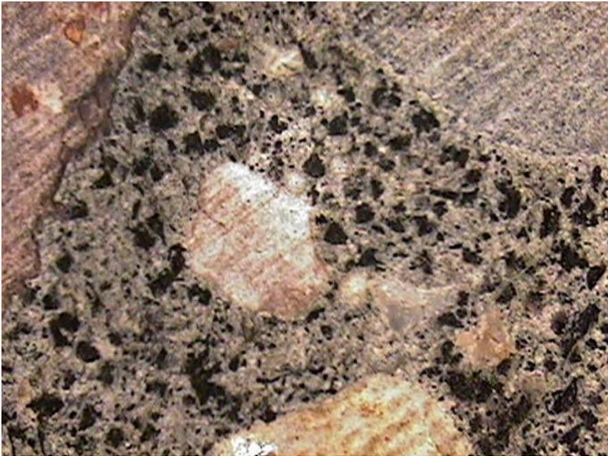
**Figure 3 Microscopic View of Crumb Rubber Distribution in a 400 lbs CR / Cyd Mix.**
