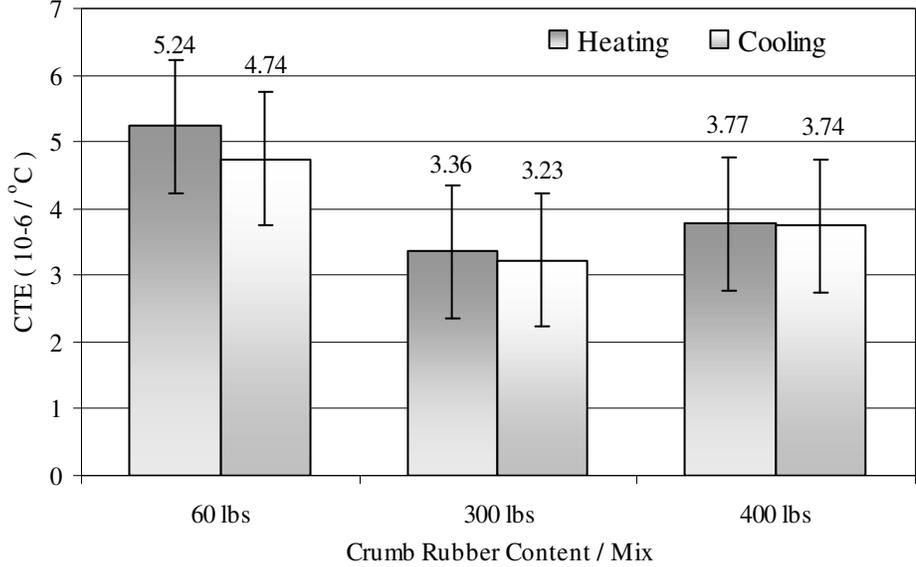
**Figure 5 Comparison of CTE as a Function of Crumb Rubber Content.**
