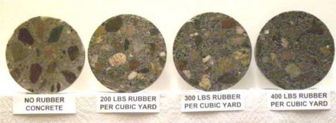
**Figure 2 Cross Sectional View of Crumb Rubber Content Variation in Trial Mixes.**
