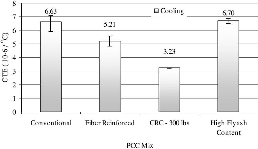
**Figure 6 Comparison of CTE for a Variety of PCC Mixes.**
