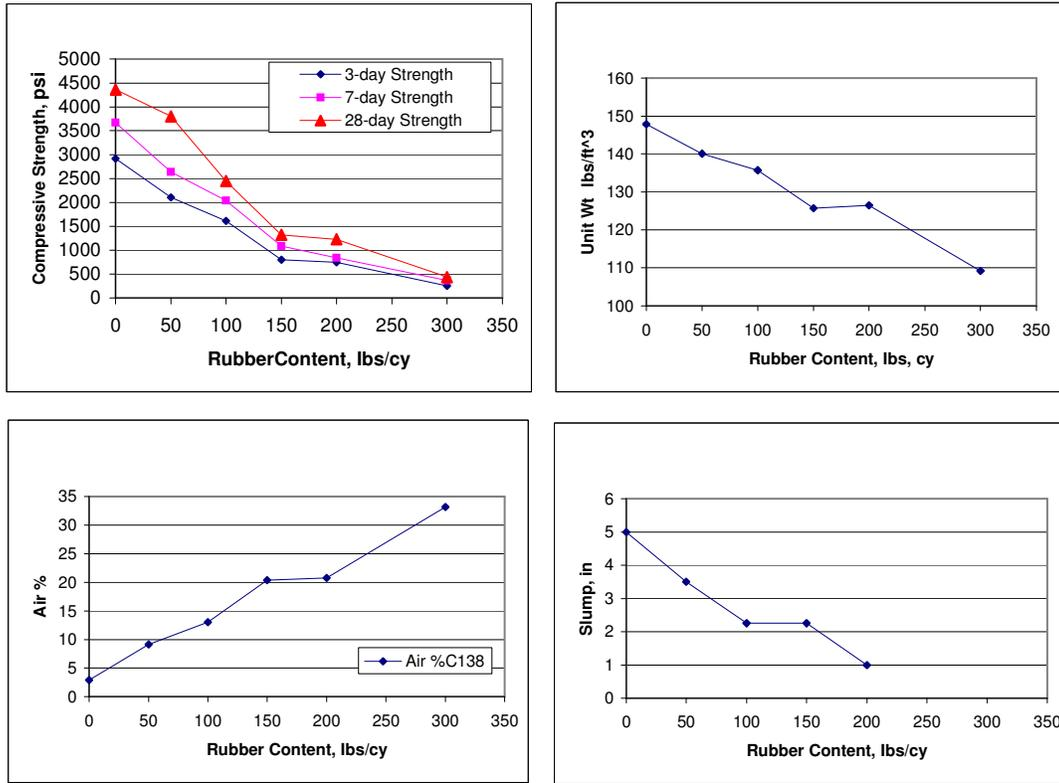
**Figure 1 Compressive Strength, Unit Weight, Air Content and Slump Variations with Rubber Content.**
