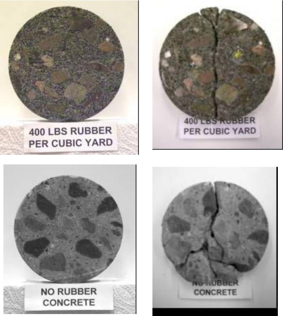
**Figure 4 Tensile Strength Failure Mechanism.**
