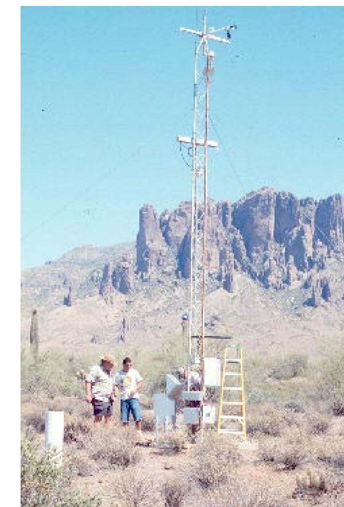
Dry deposition is measured indirectly by NOAA using air filtration from this tower at Lost Dutchman State Park ( LTER site 7). Model dry deposition rates from this site will be used to 'calibrate' deposition data obtained using LTER bucket collectors.
