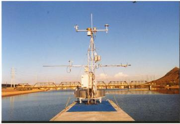
A view looking east from the west dam site of Tempe Town Lake. Automated weather station is atop a pier just above the dam and at the west end of the lake. A complete energy budget set of sensors are recording diurnal data and records are ca. two years in duration at this time.
