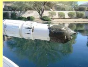
Figure 4: Lake coring device with protruding sediment
