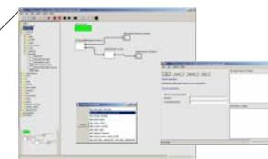
In the example to the right, the conceptual workflow described in the lower left portion of this poster is implemented with a series of actors making remote SOAP calls to web services at ADWR and MAG. The pipes between actors carry XML metadata needed to instruct each service where to find its input data and how to use it.
