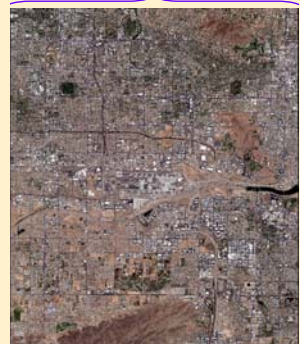
Figure 2. A true color composite of Quickbird 2.4 meter resolution data over downtown Phoenix area by displaying channel 3 (0.63 – 0.69 μm), channel 2 (0.52 – 0.60 μm), and channel 1 (0.45 – 0.52 μm) in red, green, and blue respectively.
