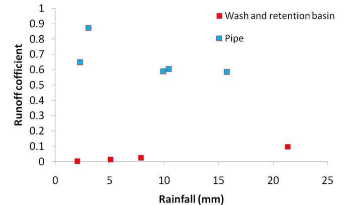
**Figure 3 (right).** Runoff coefficients for two catchments of comparable size, that differ in terms of stormwater infrastructure, for rainfall-runoff events of various sizes. The runoff coefficients is the proportion of water entering the catchment as rainfall that leaves as runoff.
