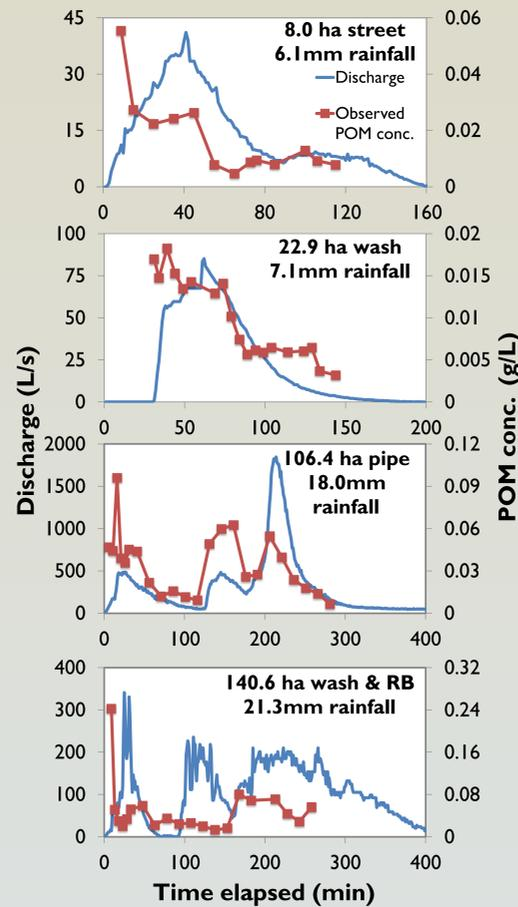
**Street drainage:** rapid transport of POM through the system, resulting in an exponential decline in POM concentration.
