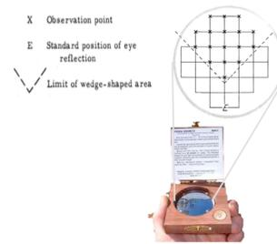
Figure 4: Densiometer with Strickler modifications.
