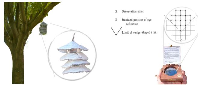
Figure 3: An iButton in its solar shield.
