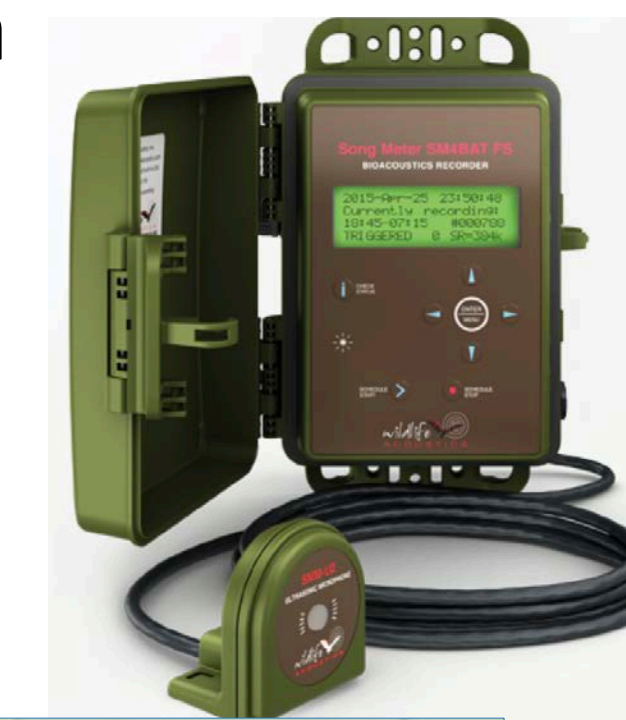
Fig 3. Wildlife Acoustics' SM4BAT-FS acoustic monitor and SMM-U2 microphone used to record bat echolocation calls.
