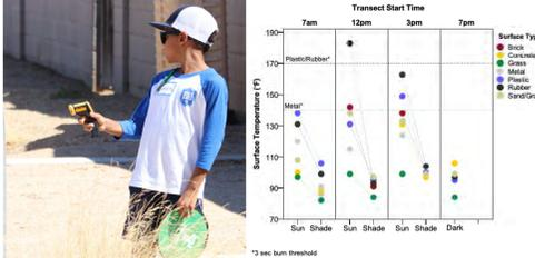
Figure 1a: Surface temperature sensor. Figure 1b: Hand-held surface temperatures ("touch-scale") at Kiwanis South Playground on August 25, 2019. Sky Harbor daytime high air temperature 103F and morning low air temperature 85F, Sunrise: 5:57 am and Sunset: 7:02 pm.
