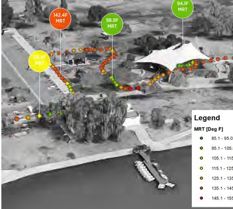
Figure 1c: Mean radiant temperatures collected using MaRTy (see figure 2a) at Kiwanis North Playground at 8am on September 12, 2019 with high at Sky Harbor of 102F and low 80F, sunrise 6:09am and sunset 6:38pm.
