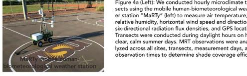
Figure 4a (Left): We conducted hourly microclimate transects using the mobile human-biometeorological weather station "MaRTy" (left) to measure air temperature, relative humidity, horizontal wind speed and direction, six-directional radiation flux densities, and GPS location. Transects were conducted during daylight hours on hot, clear, calm summer days. MRT observations were analyzed across all sites, transects, measurement days, and observation times to determine shade coverage efficacy.
