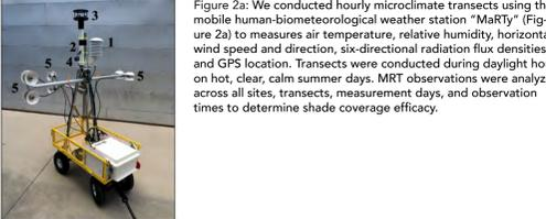
Figure 2a: We conducted hourly microclimate transects using the mobile human-biometeorological weather station "MaRTy" (Figure 2a) to measure air temperature, relative humidity, horizontal wind speed and direction, six-directional radiation flux densities, and GPS location. Transects were conducted during daylight hours on hot, clear, calm summer days. MRT observations were analyzed across all sites, transects, measurement days, and observation times to determine shade coverage efficacy.
