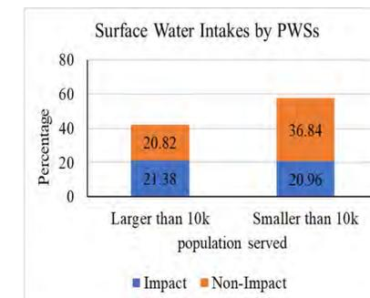
Fig 2. Number of surface water intakes non- or impacted by treated wastewater upstream categorized based upon population served by a public water system
