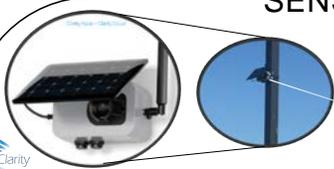
Fig 1: Clarity Air Quality Monitor: PM<sub>1</sub>, PM<sub>2.5</sub>, PM<sub>10</sub>, NO<sub>2</sub> Six locations (4x playspaces, 2x parking lot).
