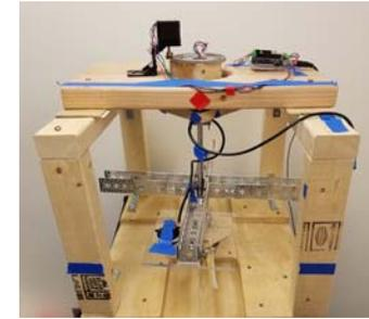
The machine has spaces for a box of water, and a release box. It rotates through these boxes and the open air to capture Carbon Dioxide.
