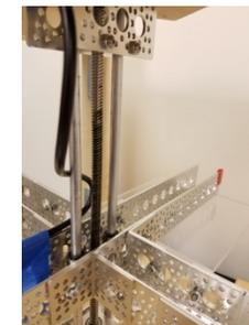
The lead screw (the dark long screw in the middle), as well as the two guide rails around it, move the arms of the machine up and down, in and out of the water and release boxes when powered by a motor.
