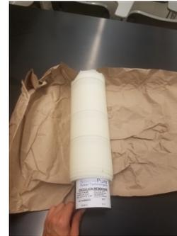
For one hour, when the sheet is dry, it will capture Carbon Dioxide, but once the sheet is dipped in water, the sheet will release Carbon Dioxide for another hour. The cycles can be repeated 1,000+ times.
